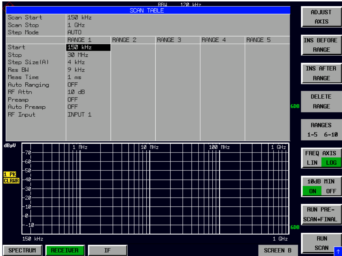
Fig. 5-3 Scan range after selecting default setup with PRESET
