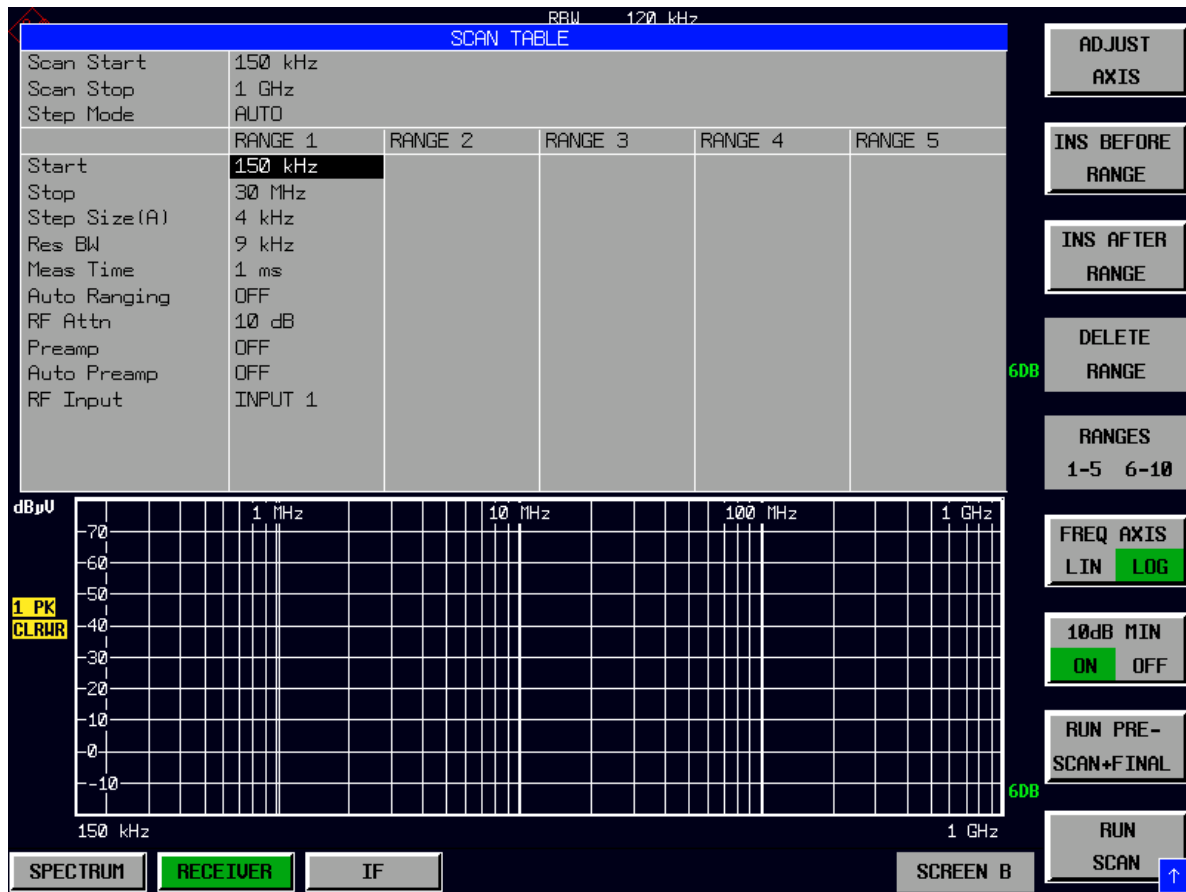
Fig. 5-4 Modified SCAN TABLE for preparing a scan
